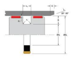
Applications with maximum radial clearance that are using nylon, phenolic, or PTFE bearings must ensure proper clearance in accordance with the bearing recommendations to avoid metal-to-metal contact. Please refer to Hallite Type 87, Type 506, and Type 533 Specification Sheets for this information.
