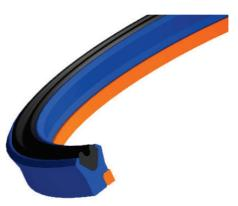
The polyacetal anti-extrusion ring extends the normal pressure range of the twin-lip design and enables the seal to withstand heavy side loads and extreme pressure spikes during operation.
