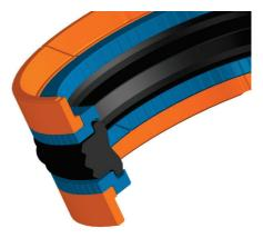
Both the L-shaped bearings and support rings are grooved to ensure that the fluid pressure properly energises the sealing element and to prevent the possibility of any pressure trapping within the seal assembly.
