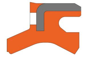
The Halite 869 is moulded in Hythane® 361, Hallite's high-performance polyurethane, for excellent durability in service.
