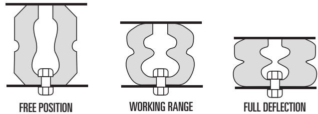
The illustration above shows the operation on an Aeon Spring in its free state, under normal working conditions and at its maximum load capacity
