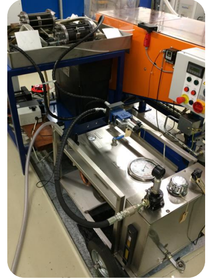
Photo 2: Pulse Test Rig
